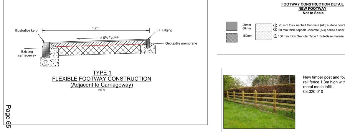
FULL HEIGHT KERB- TYPE HB2 EDGING TYPE EF (FLAT TOP) DROP KERB - TYPE BN Size 125 (w),x 255 (d) x 914 (long) Fall away from , Size: 125 (w) x 150 Size: 50 (w) x 150 (d) EF edging \_\_\_\_50 (d) x 914 (long) ∕ x 914 (long) Varies Laid flush 200mm Surface Surface Surface Upper Sub base Ipper Sub base 100 25
